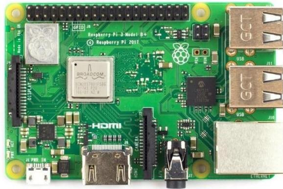
Gambar 2.1 Raspberry Pi 3 Model B+
