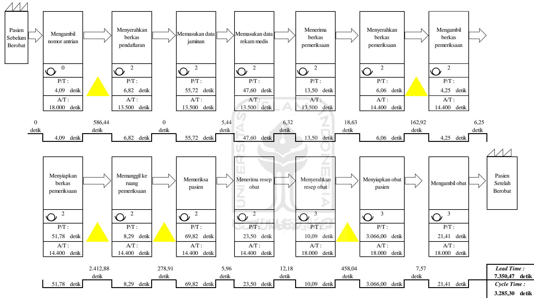
Gambar 4.9 Current State Value Stream Mapping
