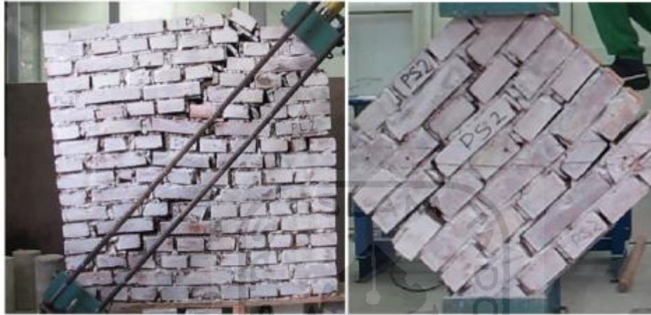
Gambar 2. 3 Pengujian Diagonal Compression Test
