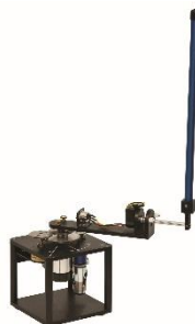
Gambar 3-16 Rotary inverted pendulum versi Quanser
