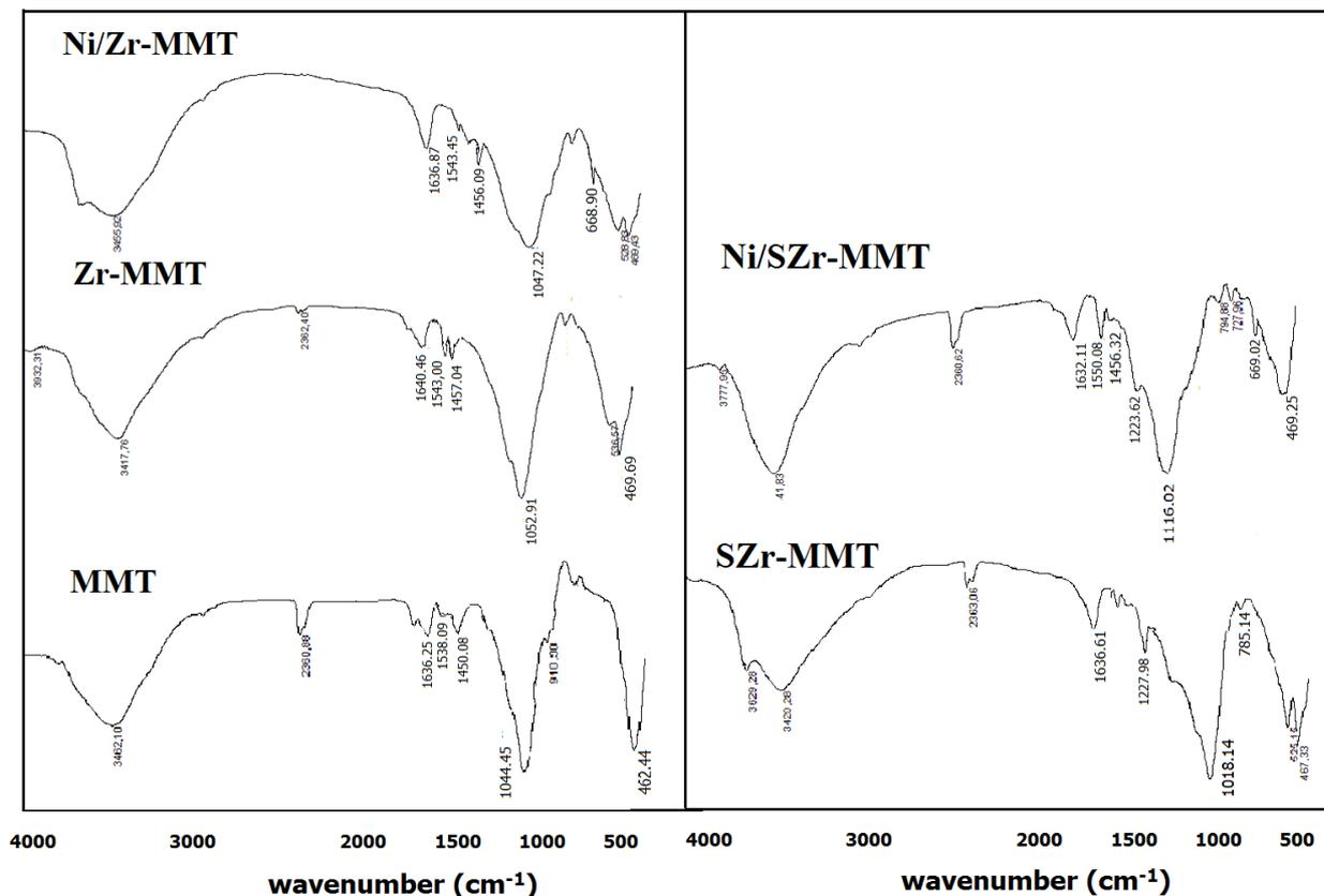
Fig. 3. FTIR spectra of pyridine-adsorbed materials.
