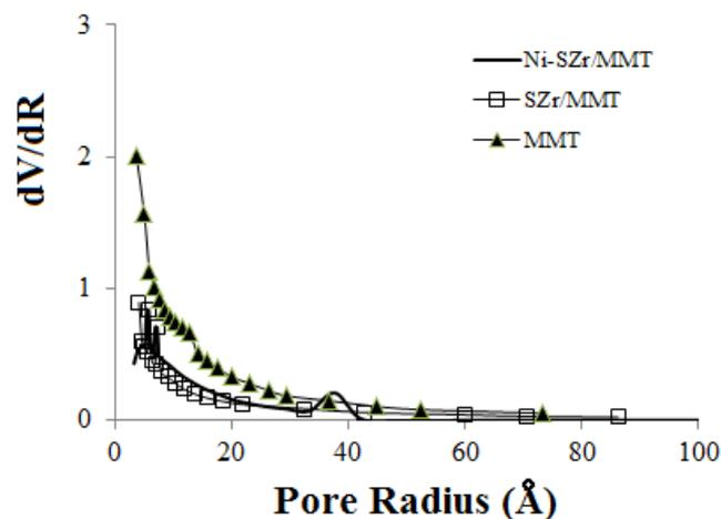
Fig. 5. Pore radius distribution of Ni-SZr/MMT compared with SZr/MMT and MMT.
