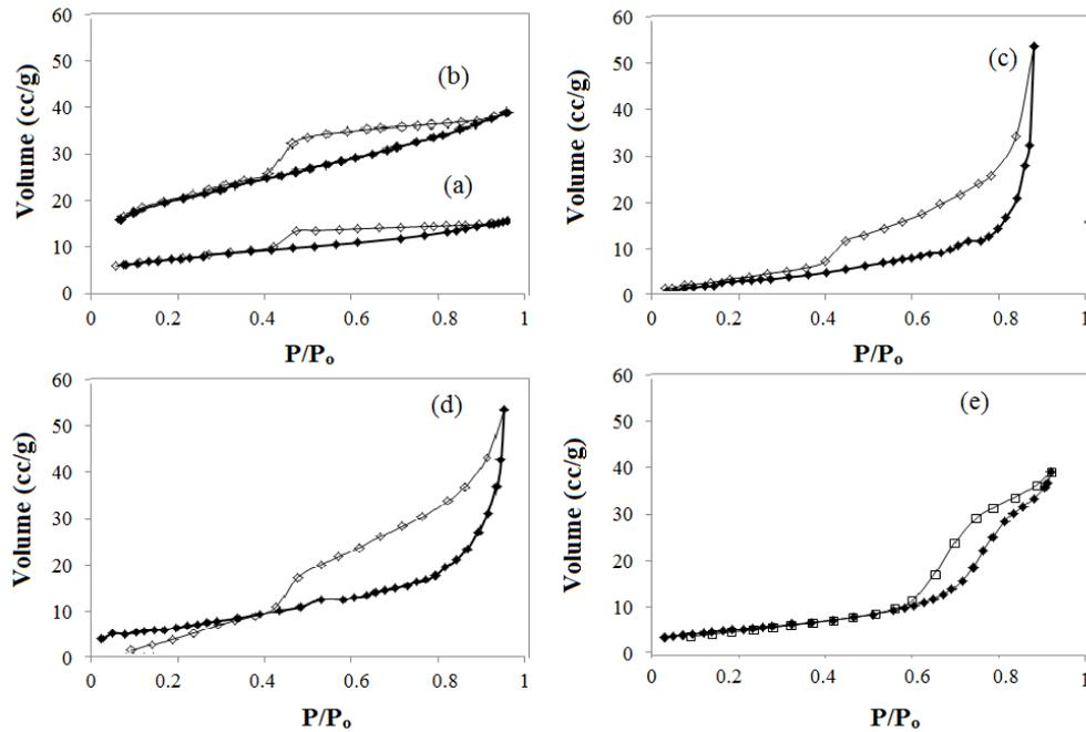
Fig. 4. Adsorption-desorption profile of (a) MMT (b) Zr/MMT (c) SZr/MMT (d) Ni-Zr/MMT (e) Ni-SZr/MMT.
