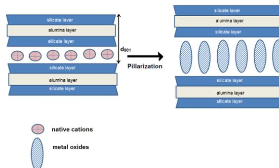
Fig. 2. Schematic representation of MMT pillarization.
