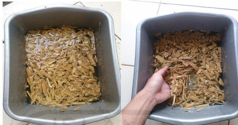
**Gambar 4.1 Proses Pencucian Bambu**
