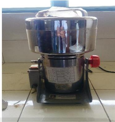
**Gambar 4.4** Proses Penghalusan Bambu (blender)
