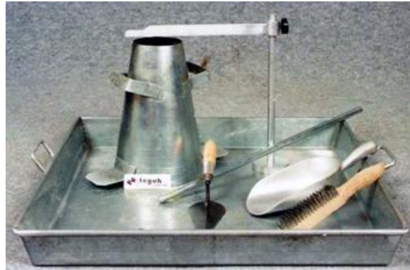
Gambar 4.12 Slump test set
