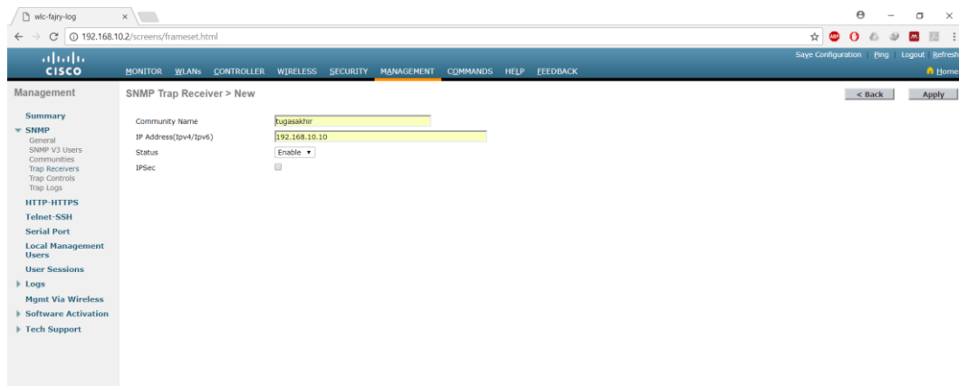
Gambar 5.1 Setting Trap Receiver WLC
