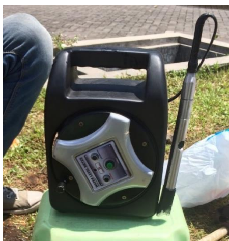
Gambar 5.10 Alat Water Level Meter
