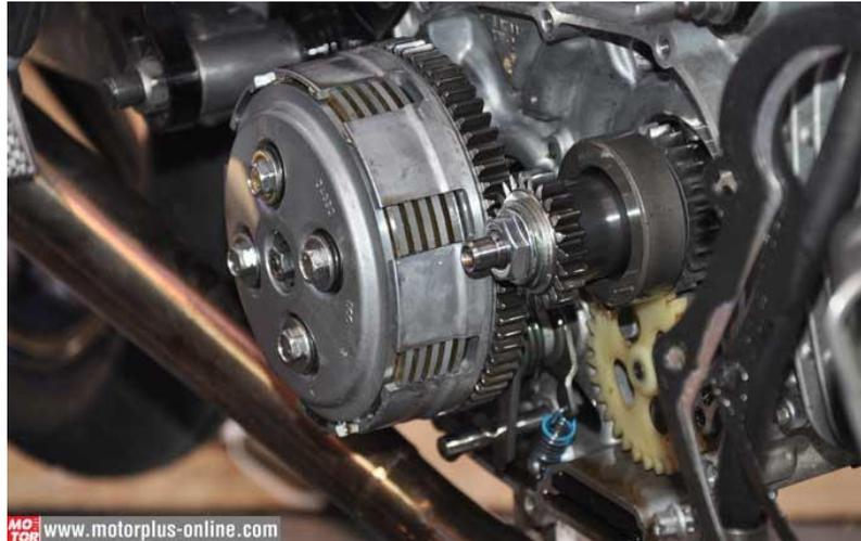
Gambar 2.1. Kopling Sepeda motor
