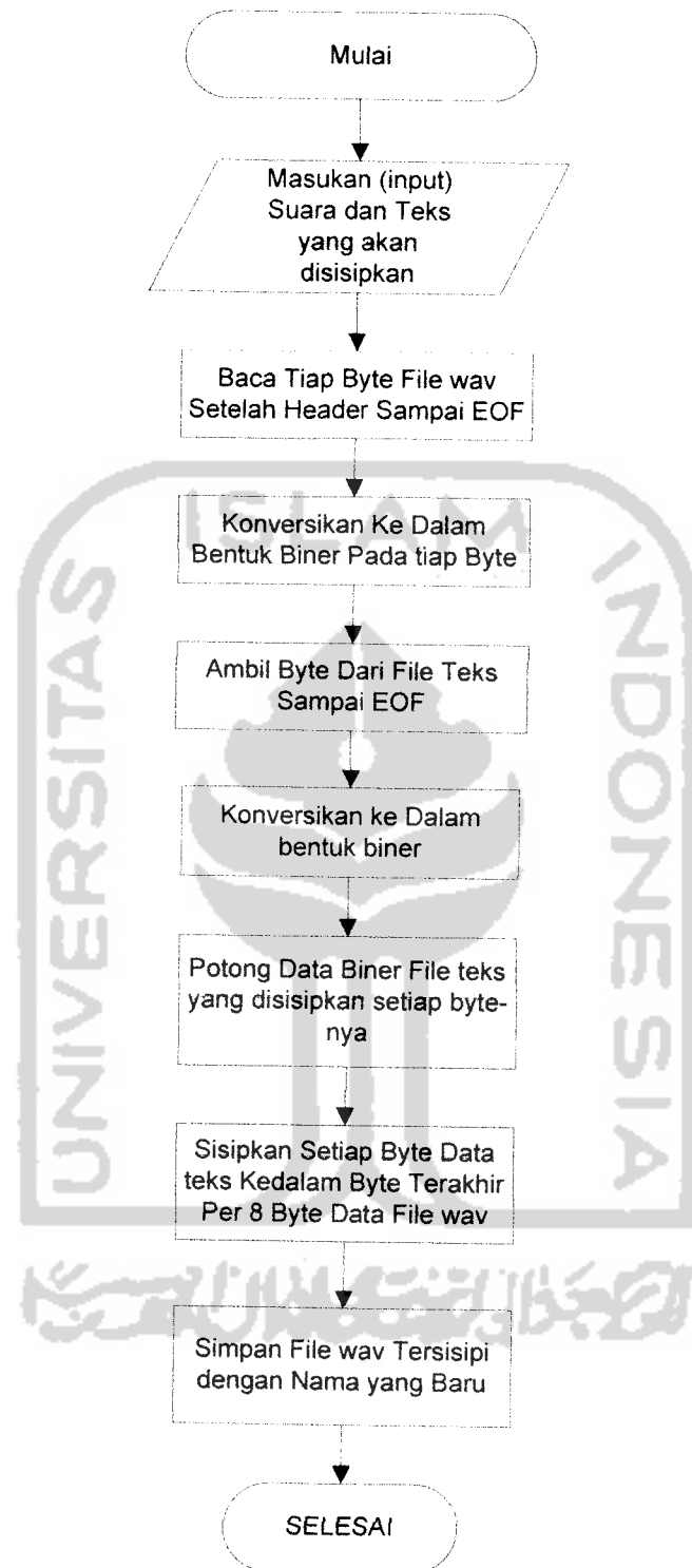
Gambar 4.2 Diagram FlowChart Proses Penyisipan File Teks
