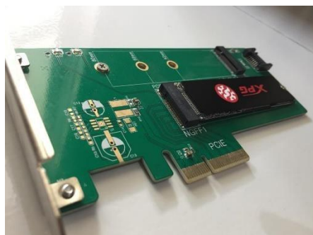
Gambar 4.3 Converter SSD M.2 NVMe Adata XPG SX6000 Lite
