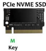
Gambar 2.5 Connector SSD M.2 Slot NVMe
