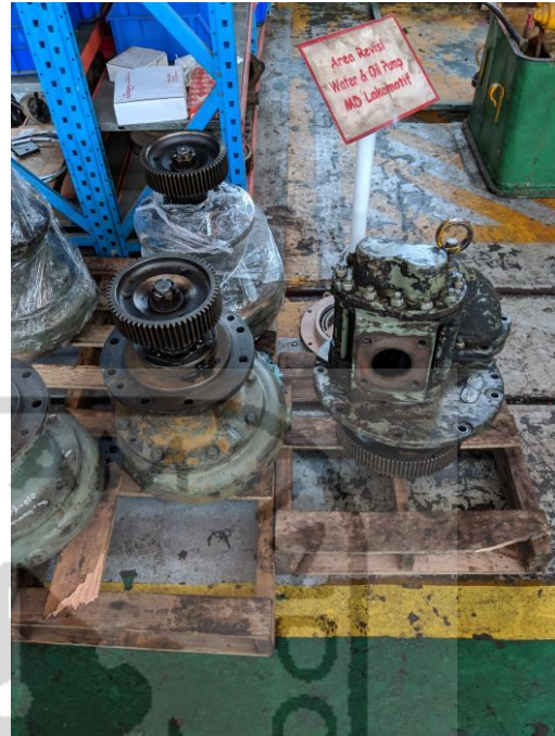
Water pump dan oil pump
