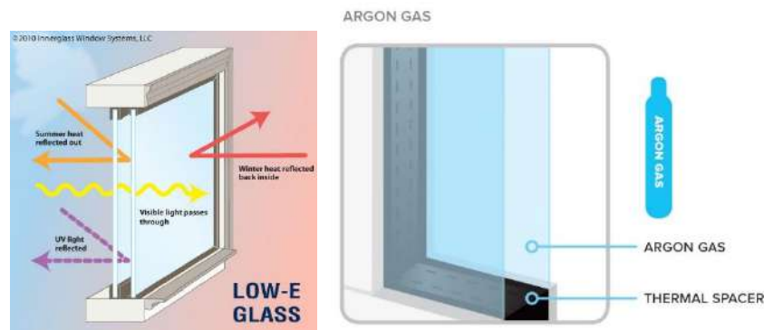
Gambar 2.29: Kaca Double Low-e & Gas Argon
