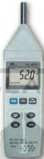
Gambar 3. 4 Sound Level Meter (Sumber : www.wikipedia.com )
