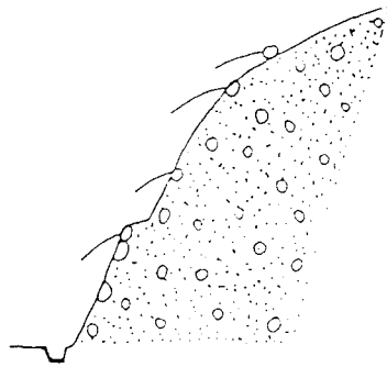
3.1.c. Failure due to accelerated weathering caused by cutting
