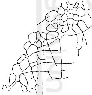
3.8.a. Rock with progressed joint/crack
