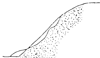
3.1.a. Surface erosion due to dry wet weather, rainfall
