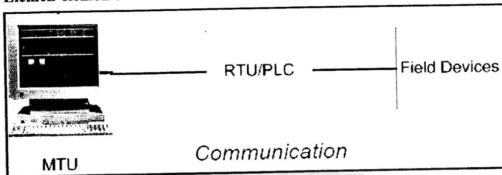
Gambar 2-8 Elemen – elemen SCADA
