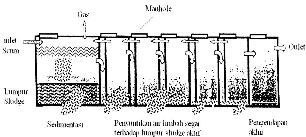
Gambar 3.4. *Septic tank susun* (Sasse, 1998)
