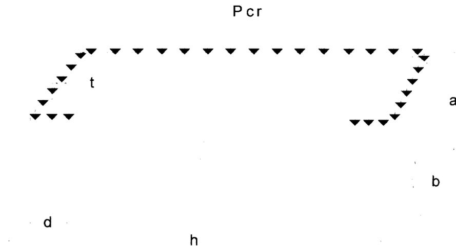
**Gambar 3. 6** Profil *Lipped Channel*
