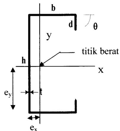
**Gambar 3.12** Profil *Lipped Channel*
