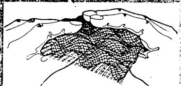
TENSAR MAT For dry & intermittently wetted slopes Polymer = polyethylene. Thickness: 8 mm. Weight = 0.45 kg/m 2 . Tensile Strength: 3.2 kN/m. Roll dimensions: 30 m x 4.5 m (30 m x 1.5 m and 30 m x 3.0 m rolls are available to order)
