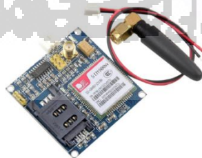
Gambar 2. 4 Tampilan Modul GSM SIM900A
