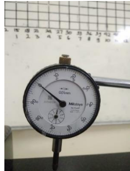
Gambar 4.3 Dial Indicator Mitutoyo
