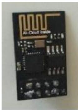
Gambar 4. Modul ESP-8266
