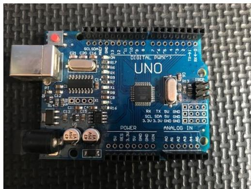
Gambar 2.1 Modul Arduino Uno
