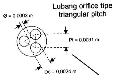
Lubang orifice tipe triangular pitch
