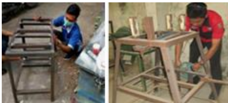
Gambar 2. Finishing rangka & setting
