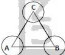
$$\text{Luas ABC} = \frac{1}{2} \times AB \times \text{Pitch} \sin 60^\circ$$
