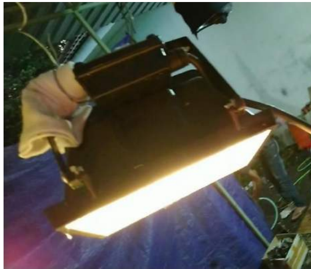
Gambar 4. 5 Lampu Tembak Cat Oven
