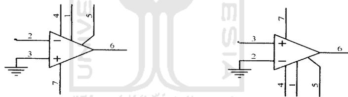
( a ) *Op-Amp inverting* ( b ) *Op-Amp non- inverting*
