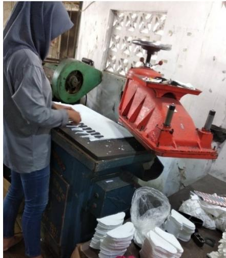
Gambar 4. 3 Proses Press Cutting
