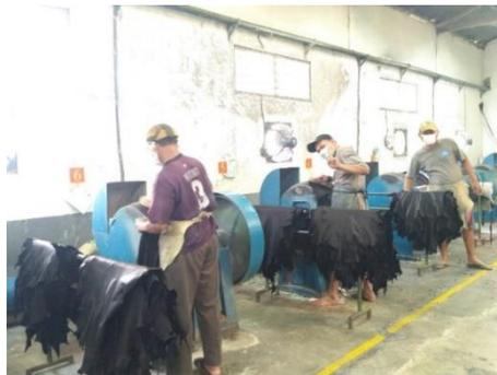
**Gambar 4. 11** Proses *Stacking*
