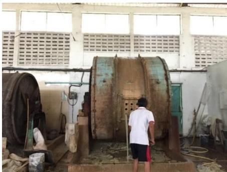
**Gambar 4. 21** Proses *Liming*
