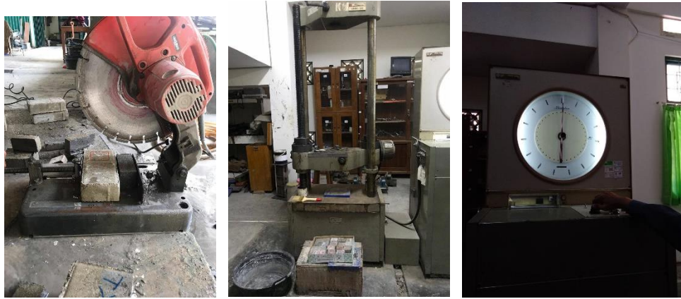
Gambar 3.6 Uji Kuat Tekan Paving Block
