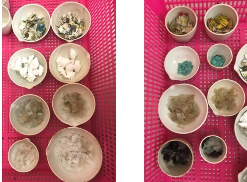
**Gambar 4. 4.** Sampel Hasil Oven di suhu  $105^{\circ}\text{C}$
