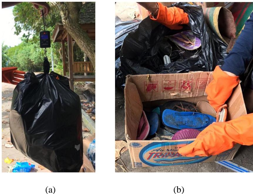
**Gambar 4. 2.** (a) Penimbangan Sampel, (b) Pengukuran Volume Sampel
