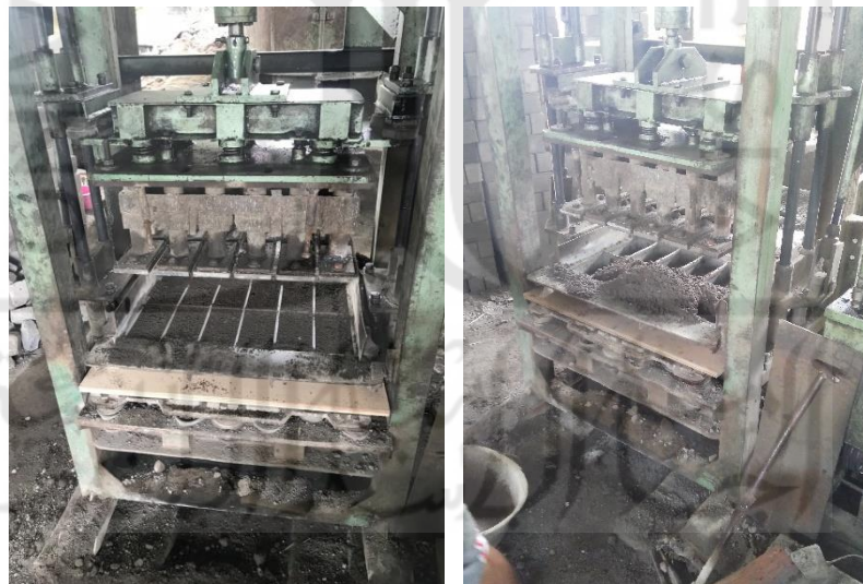
Gambar 3. 6 Proses Pencetakan Paving Block
