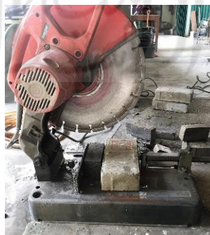
Gambar 3. 8 Proses pemotongan Paving Block
