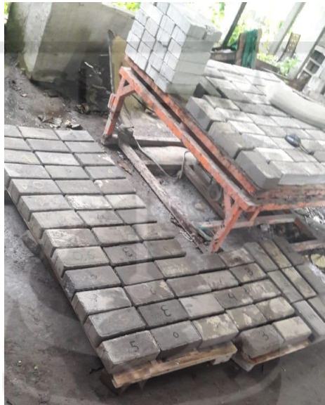
Gambar 3. 7 Proses Perawatan Paving Block
