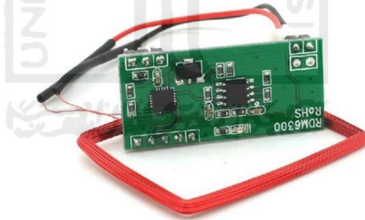
**Gambar 2.4** Modul RFID RDM6300 (“Amazon.com: Generic 125 KHZ EM4100 RFID Card Read Module RDM630 (UART) Compatible Arduino: Toys & Games,” n.d.)
