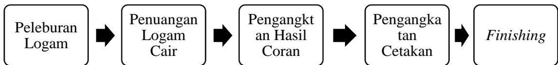
Gambar 4. 2 Proses Pengecoran Aluminium
