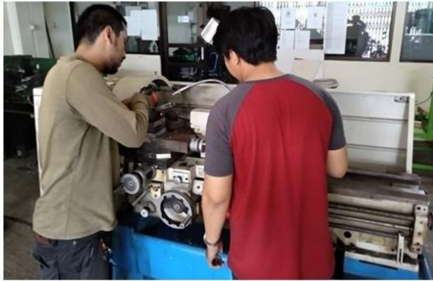
Gambar 3.31 Proses pengelasan rotary friction welding
