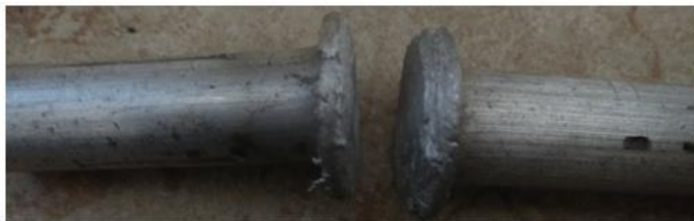
Gambar 4.2 Hasil sambungan pengelasan rotary friction welding gagal
