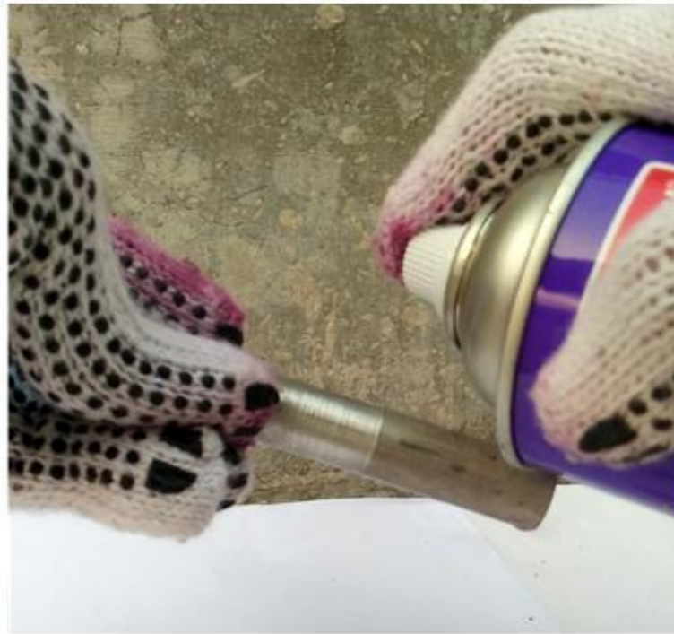
Gambar 3.32 Pretreatment dye penetrant
