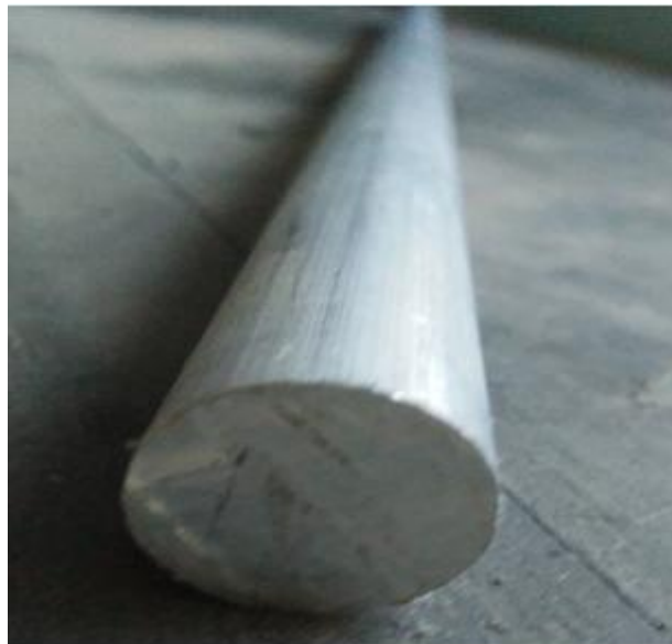
Gambar 3.2 Aluminium seri 4017 diameter 16mm
