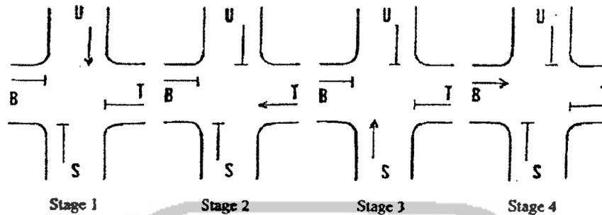
Gambar 2.2 Diagram pengaturan “stage”
