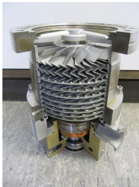
Gambar 2.3 Momentum Transfer Pump (Kleinsatelliten, 2014)
