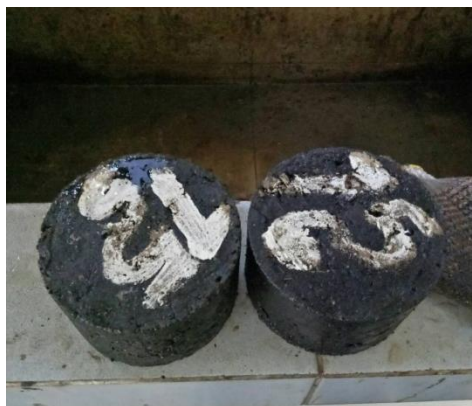
Campuran LASTON AC-WC
