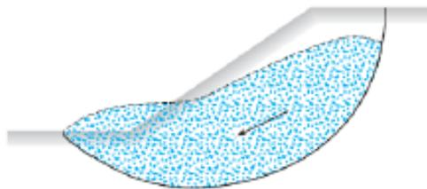
**Gambar 3.2 Keruntuhan Lereng Slide**
