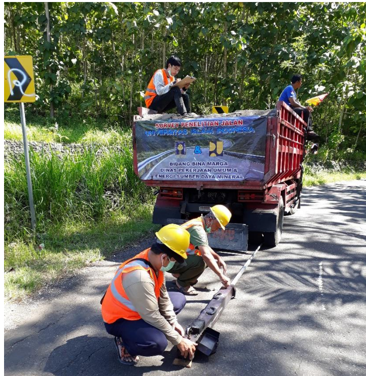
Gambar L-4.6 Uji Lendutan Balik ( Benkelman Beam )
