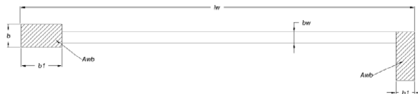
Gambar 3.30 Dimensi Minimum Struktur Dinding (Paulay & Priestly, 1992)
