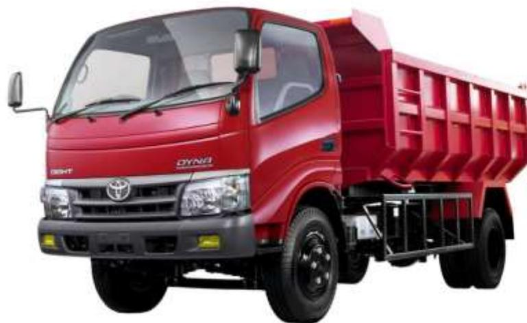
**Gambar 3.3** *Dump Truck* kapasitas bak 7 m<sup>3</sup>
