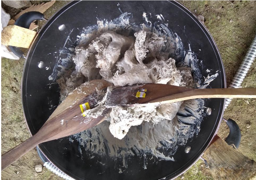
Proses pelelehan plastik polypropylene bekas
