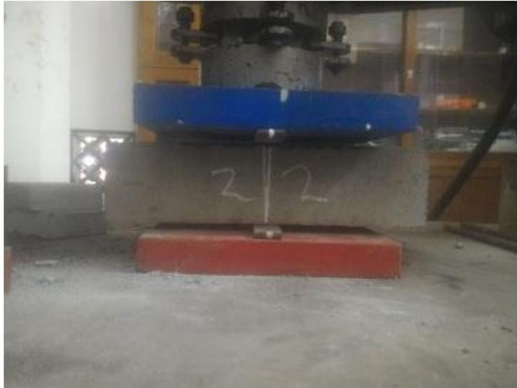
**Gambar 4.7 Uji Tarik *Paving Block***
