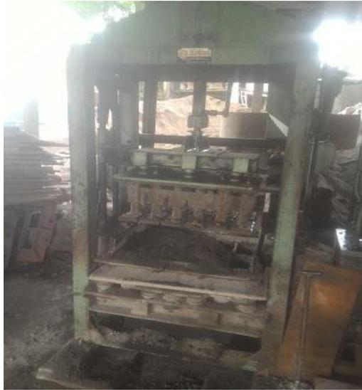
**Gambar 4.2 Mesin *Press Paving Block***
