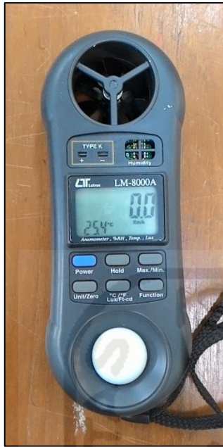
Gambar 5. 4 in 1 meter tipe LM-8000A
