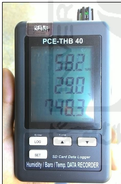
Gambar 3. Barometer tipe PCE-THB 40
