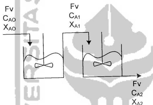
$$V_1 = \frac{Fv.(X_{A1} - 0)}{k.C_{A0}(1 - X_{A1})(M - X_{A1})}$$
