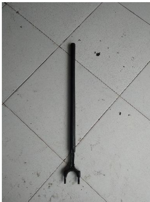
Gambar 3.11 Pegangan Kayuhan Poros Engkol
