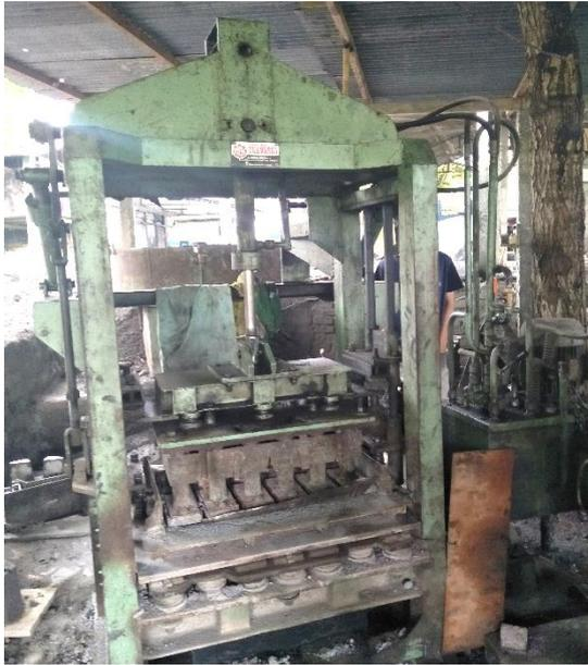
**Gambar L-1.7 Mesin Cetak *Paving Block***
