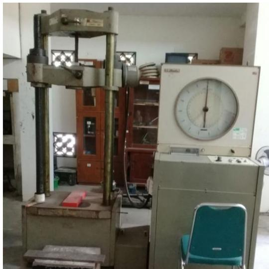
**Gambar L-1.10 Mesin Uji Kuat Tarik Belah *Universal Testing Machine*
