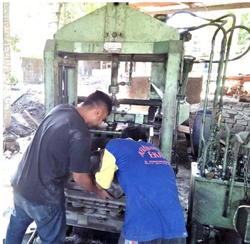
**Gambar L-4.2 Proses Pencetakan *Paving Block***
