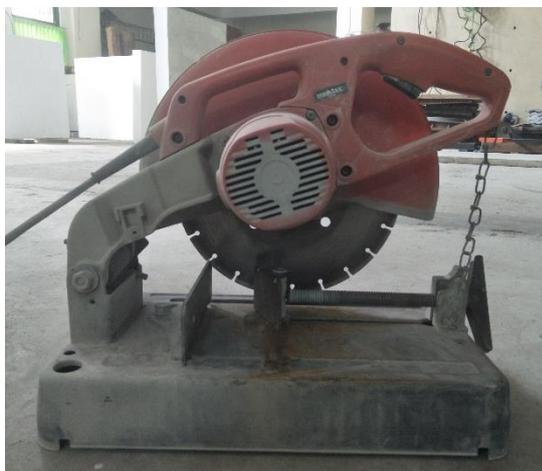
**Gambar 4.9 Alat Pemotong *Paving Block***
