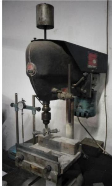
**Gambar L-1.11 Mesin Uji Keausan *Soiltest, INC***
