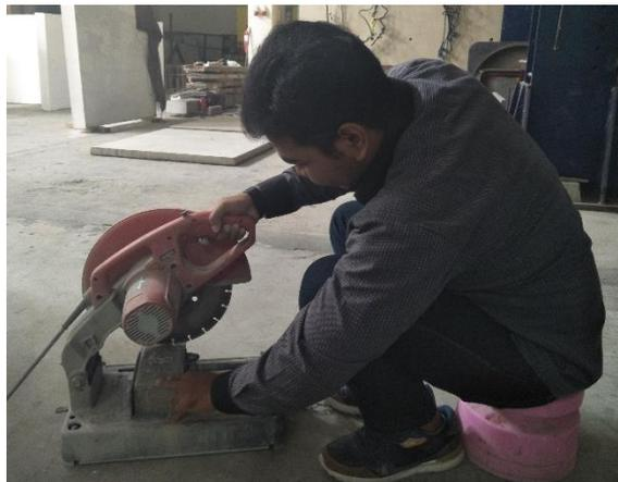
**Gambar 4.23** Proses Pemotongan *Paving Block*
