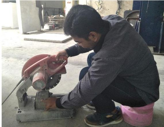
**Gambar L-4.4** Proses Pemotongan *Paving Block*
