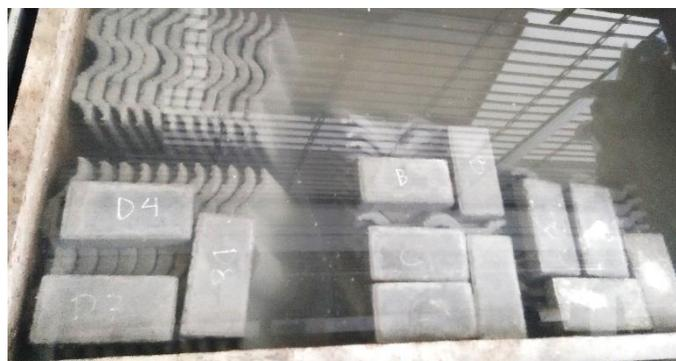
**Gambar L-4.3 Proses Perawatan *Paving Block***
