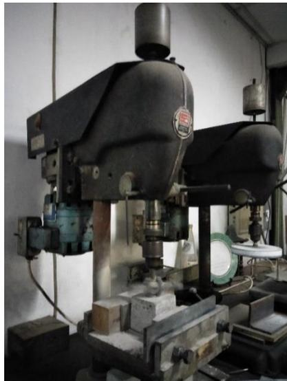
**Gambar 5.4 Pengujian Keausan *Paving Block***
