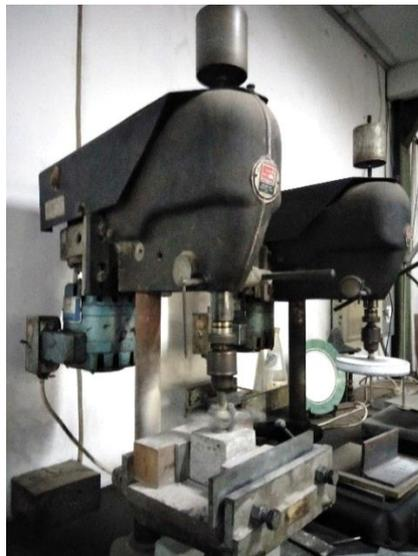
**Gambar L-5.2 Pengujian Keausan *Paving Block***
