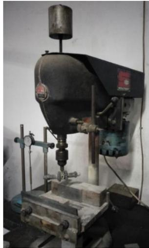
**Gambar 4.12 Mesin Uji Keausan *Soiltest, INC***
