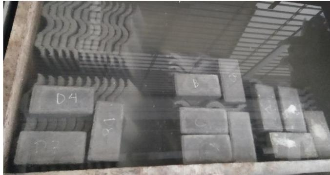
**Gambar 4.22** Proses Perawatan *Paving Block*
