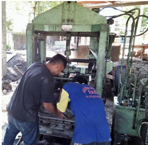
**Gambar 4.21** Proses Pencetakan *Paving Block*
